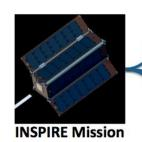
**Low-Cost Heliophysics:** Constellation of 50 standalone 10 kg spacecraft to monitor the solar wind 3D structure at Sun-Earth L1.
