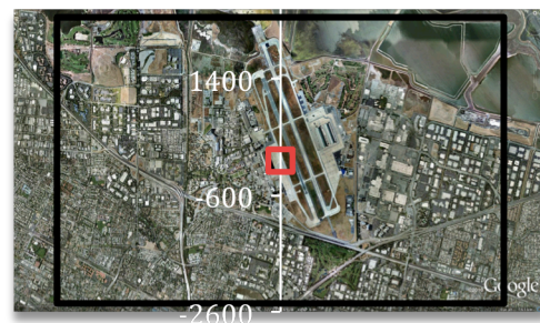
Figure 2: FOV simulation of a 152.4 mm f/8 telescope front end to a Canon EOS 5D Mark II sensor (Pixel size of 6.4 \mu m and a resolution of 5616 by 3744 pixels) in a 250 km orbit.
