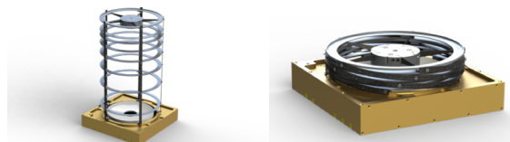
Figure 7: Rendering of mechanical structure (minus light shroud) shown deployed above and collapsed below.
