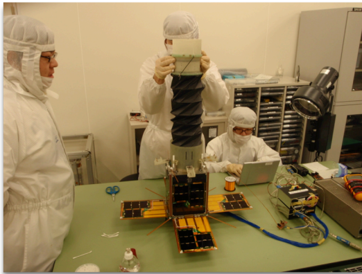
Figure 4. University of Tokyo PRISM team member assembling the PRISM space telescope [2].
