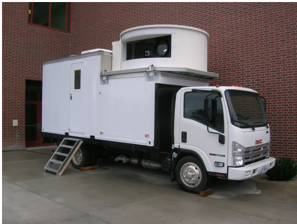
Figure 1. The VISSTA van. The ELT aperture can be seen at the right side in the turret behind the cab.
