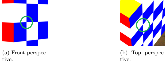
Figure 1: Examples of potential Harris feature points on a checkered cube from different perspectives.
