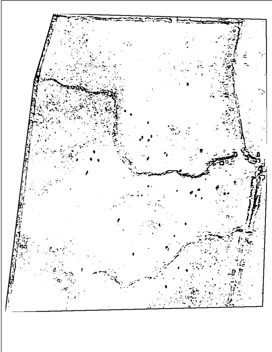
Figure 3.12. Image resulting from the subtraction of the first principal component and a simulated background image, followed by the Rosin corner thresholding method.
