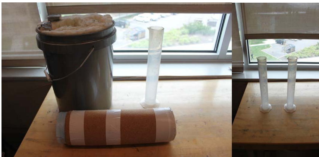
Figure 5-12. Experimental outer and inner containers with insulation.
