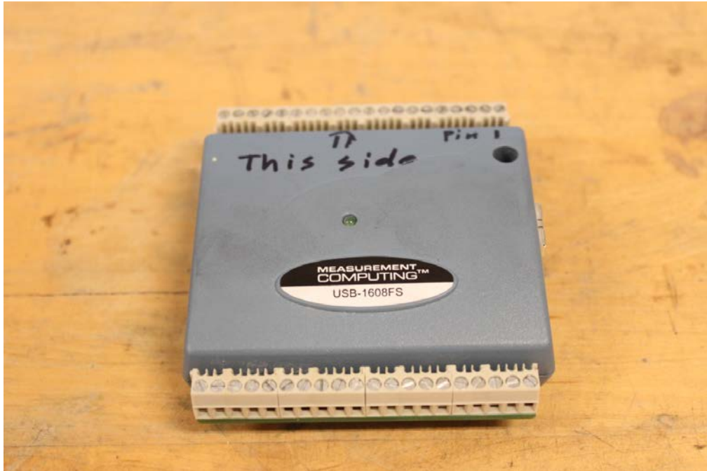
Figure 5-11. Experimental voltage DAQ measurement computing USB 1608FS.
