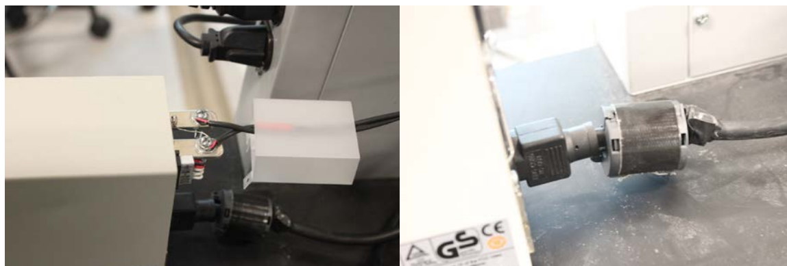
Figure 5-7. Constant current contact points for power supply, induction collar also featured.
