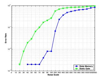
Fig. 2: Simulated error rate results obtained using the  $0.6\mu m$  CMOS model in Virtuoso Spectre.
