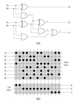
Fig. 5: Implementations of a two-bit binary adder function, representing a traditional ripple-carry design (a), and a crossbar design suitable for some nanoelectronic device families (b). The ' $\star$ ' symbol indicates the occurrence of an error which propagates to multiple signals.
