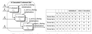
Fig. 1: Local implementation of a variable node.
