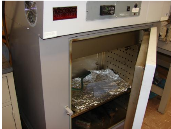
Fig. 2.9: Oven for curing the printed antennas.
