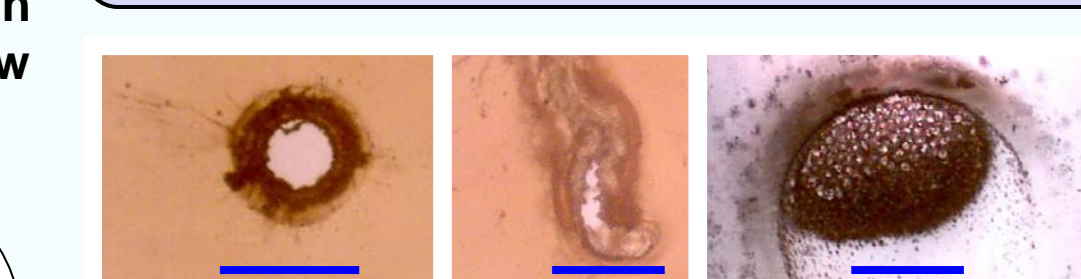
Fig. 7. Images of breakdowns. Kapton E usually breaks down with circular holes (left), while LDPE is more irregular (center). ePTFE can breakdown rather spectacularly (right).
