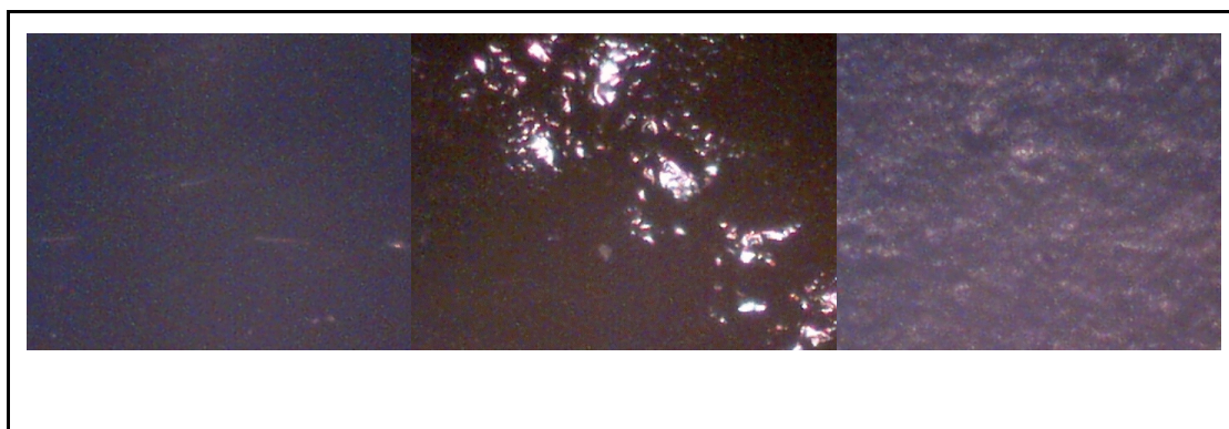
FIG. 5.3: Optical microscope pictures of HOPG (left), g-C (middle), and colloidal graphite (right). The images are 1 mm across. The magnification is approximately 50:1.
