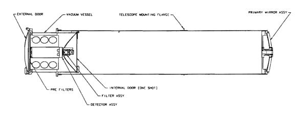
Figure 3. Layout of the SWATH high resolution X-ray instrument.
