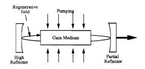
Figure 3 - A generic laser oscillator.
