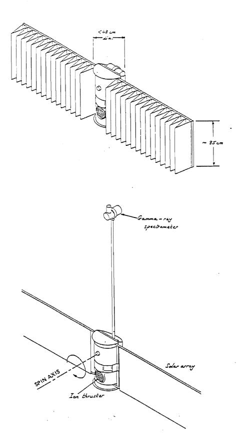
JPL's Proposed LGAS Spacecraft would be launched as a compact cylinder and would then unfurl large solar arrays to power its two ion thrusters
