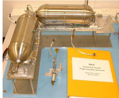
Figure 7: The propulsion system installed on the satellite to perform semi major axis corrections
