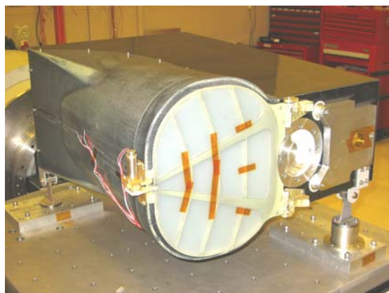
Figure 7 Camera flight structure qualification
