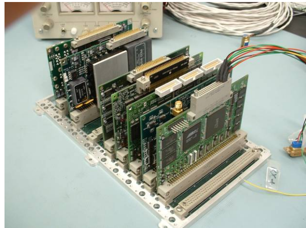
Figure 8: The IRIS spacecraft processing is based on a low-power computer developed for USUSat II.
