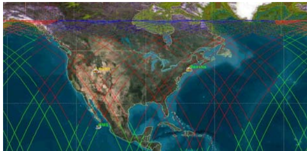
Figure 7: As illustrated by this coverage map, the use of ground stations in Logan, UT, and Boston, MA, gives IRIS sufficient coverage to downlink an average of 65 uncompressed images per day.
