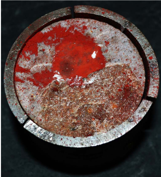
Figure 11. Stationary quartz sandstone core. Fracture is from failure under uniaxial compression. The hematite gouge is bright red. Core is housed in a notched steel pipe.
