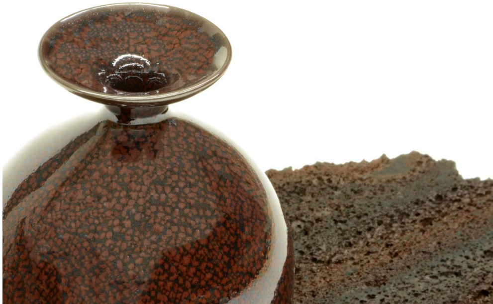
Figure 8. Ceramic work by M. Fiske (left). Base glaze substrate to (right). Glaze created from 25% basalt and 75% rhyolite.
