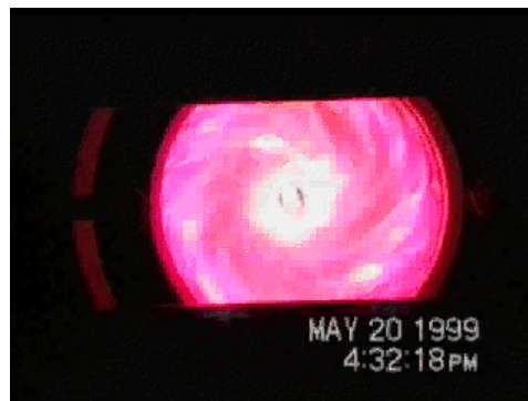
Fig. 9 VFP combustion seen through a Plexiglas fuel grain (with a UV filter)
