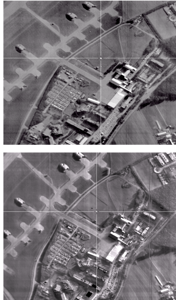
Fig 2. – Airborne experiment results: hot plate of 1m 2 with 200°C (cross marked) detected from 3000 m altitude. MWIR-image above, LWIR below
