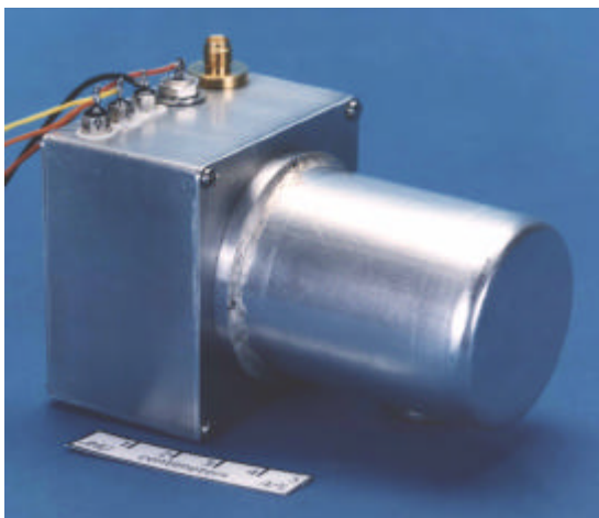
Figure 9. Miniaturized ultrastable oscillator development model with TOPEX-quality stability.
