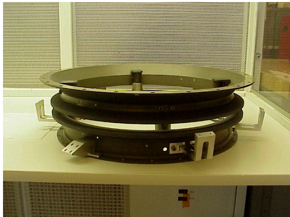
Figure 4. Primary structural components for the ESPA application.
