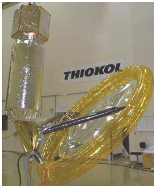
Figure 2. Subscale STP Deployment Test
