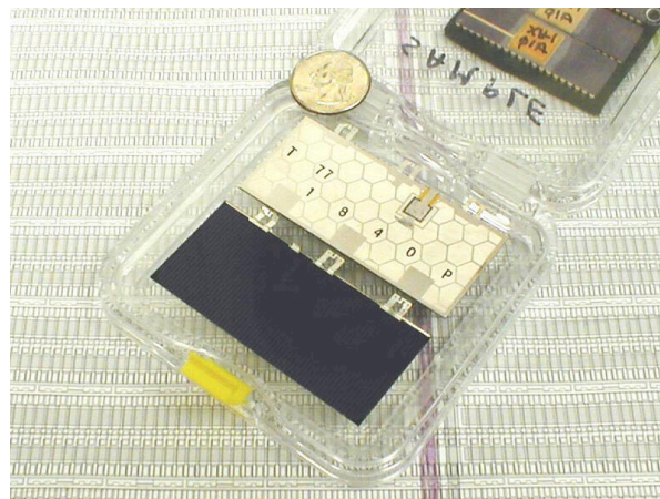
Fig. 5—A sample of two of the GaAs/Ge solar cells. The front (darker) and back of the cells are shown.
