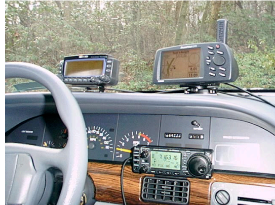
Photo 4. Chas Richard, W4HFZ's mobile APRS Satellite capability (including HF). With an APRS Satellite, he can send and receive brief text messages anywhere on the planet a few times a day.
