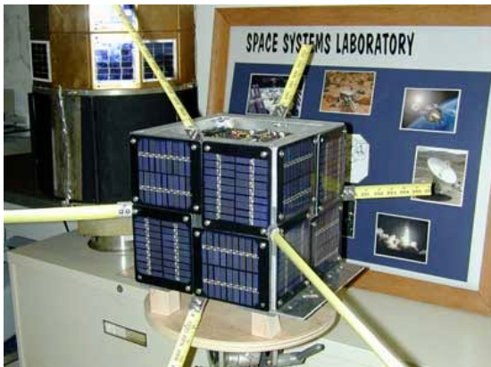
Photo 2. Personal Communications Satellite (PCsat) with Antennas
