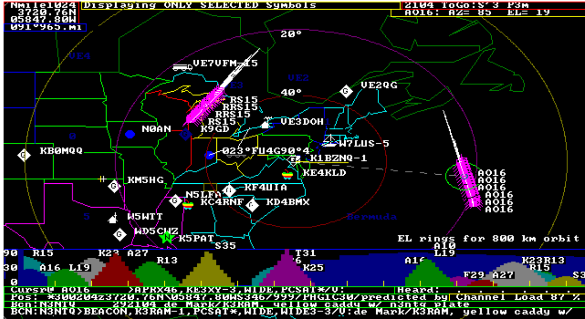
All satellites are shown on the map as moving objects. Across the bottom of the screen the next 2.5 hours of satellite passes are shown in a graphic showing the maximum elevation of the pass.
