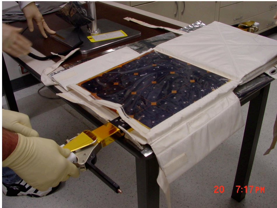
Figure 7: The “pizza box” is shown unfolded with the arrays inserted. Note the transparent “window” for inspection prior to removal from the package. The long pouch unfolded at the bottom of the picture (one of two) was used for storing the probes. This entire assembly was fastened to the outside frame of the FPP and provided a convenient single package for the Crew to transport on EVA.
