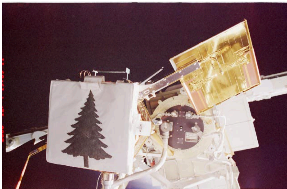
Figure 8: This is a photo taken of the FPP after installation on the ISS showing the back side of the “pizza box” assembly used for carrying the solar arrays and probes to the work site. The “Christmas tree” is not a standard feature. The back side of one solar array and the dogbone handle for the BRT interface are also clearly visible. The large cylinder in the background is the solar array canister.
