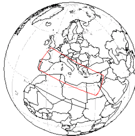
Figure 9. A 10 min. observation period would cover the entire Mediterranean (red rectangle) when looking sideways from a 30° inclined orbit.
