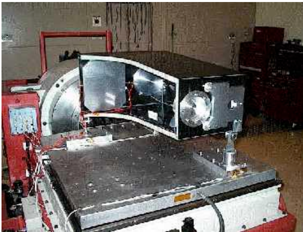
Fig 3 Engineering model undergoing vibration testing
