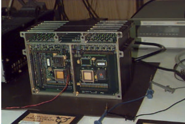
Figure 7. Picture of mechanical assembly used in vibration and thermal-cycle tests
