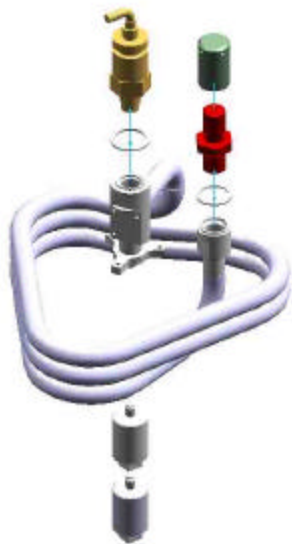
Figure 6 : Exploded view of propulsion assembly
