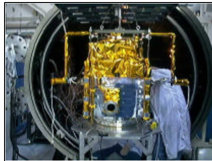
Figure 18. Thermal vacuum testing
