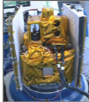
Figure 19. Confidence vibration testing
