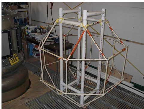
Figure 2. Magnetic field simulator to be used for lab testing the student's magnetometers.
