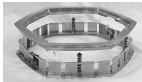
Figure 8: Intersatellite/ Lightband Separation System.
