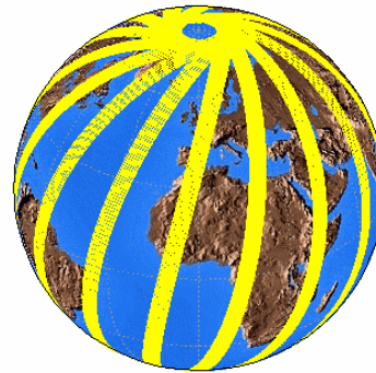
Figure 6 Daily Imaging Coverage of a 600km Swath (Descending Pass)
