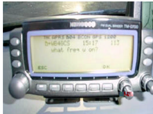
Photo 6. The front panel of the TM-D700 showing an incoming 15 byte message (Messages can be longer up to 64 bytes).
