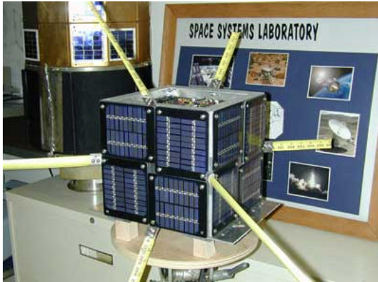
Photo 1. Prototype Communications Satellite (PCsat) with Antennas
