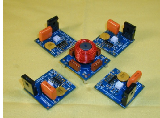
Figure 3 Vacuum Arc Thruster PPU designed for use aboard ION, Open View
