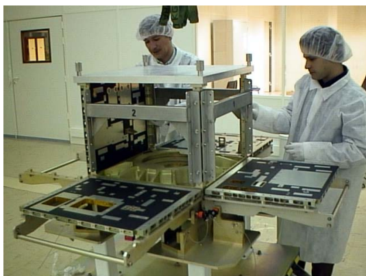
Figure 12 : MYRIADE platform structure
