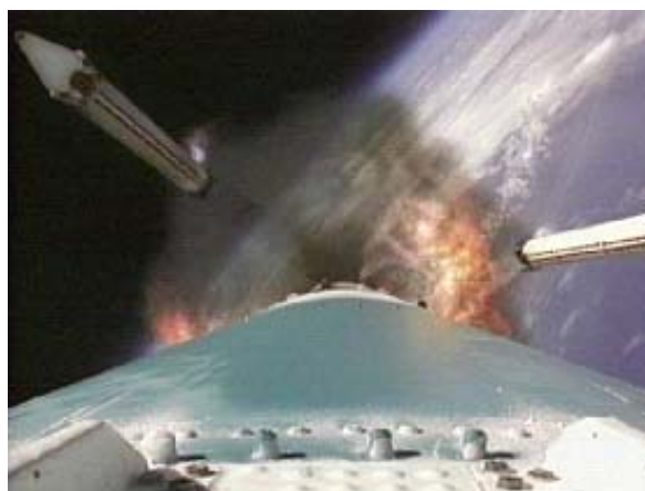
Figure 1. RocketCam View of Delta II SRM Sep.
