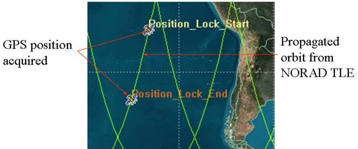
Figure 20: GPS Position Estimation: GPS estimated positions plotted relative to TLE estimated ground track
