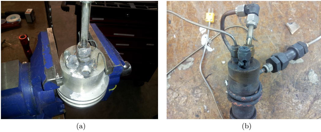
Fig. 5.24: Forward enclosure and decomposition igniter after the failed forward enclosure test.
