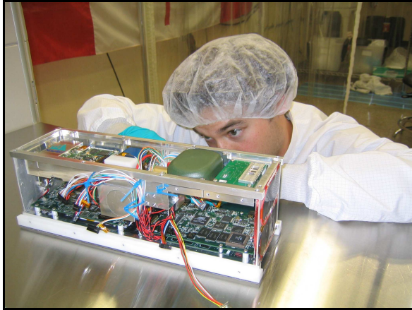
Figure 1: CanX-2 being assembled in the SFL clean room.
