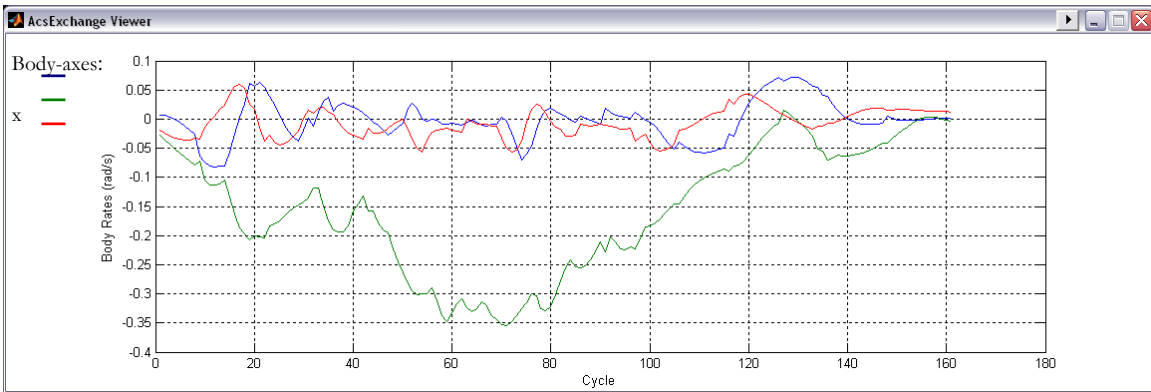
Figure 17: EKF estimated body-rate plot during wheel spin-up
