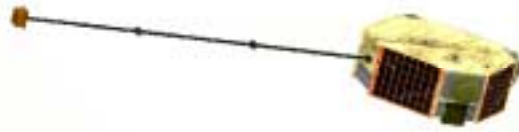
Figure 5. Impression of vehicle during science flight with magnetometer boom deployed.
