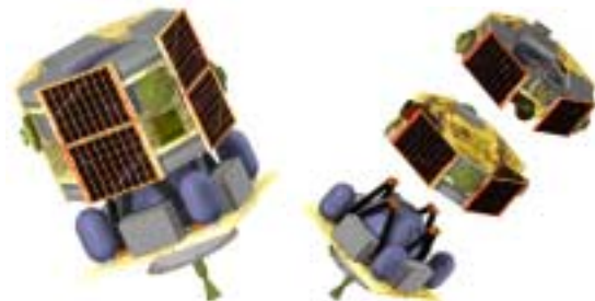
Figure 2. Multiple spacecraft adaptor and dispenser
