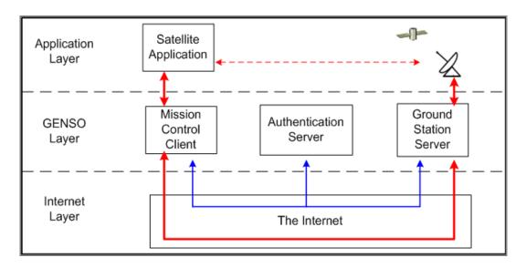
Figure 1: Layer Model of the GENSO System
