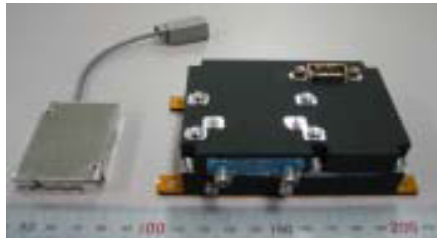
Fig.1: Left : Automobile-Navigation GPS Receiver CCA-370HJ, Right : Flight Model with RF Hybrid for INDEXT Satellite
