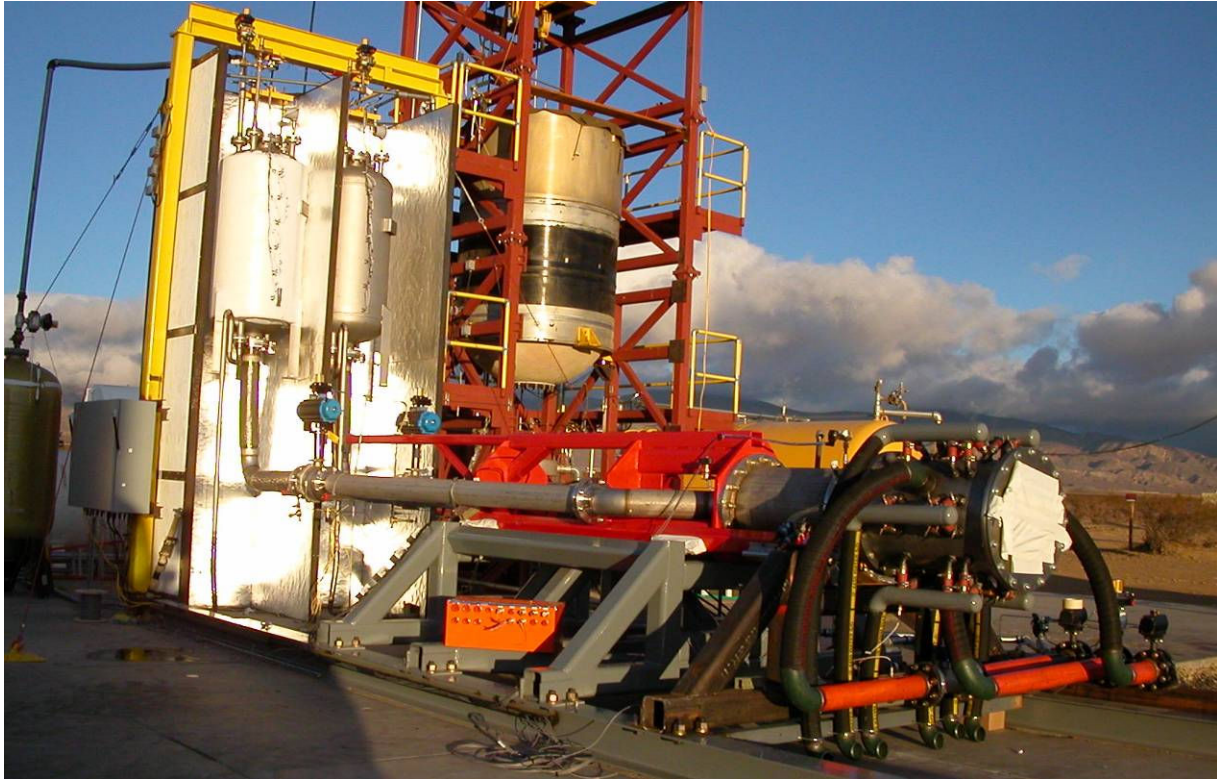
AirLaunch passed the Horizontal Test Stand (HTS) Readiness Review Milestone in early 2008. The new HTS is on the left; the Vertical Test Stand is on the right, shown with the flight-weight Integrated Stage 2 test article used in Phase 2B.
