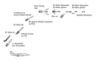
Figure 11. Three-Stage SpaceSpike-1 Flight Sequence
