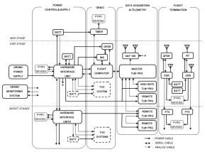
Figure 14. System Block Diagram of Miniaturized and Low-cost Avionics
