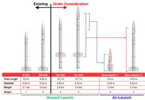
Figure 5. SpaceSpike Heritage from S-520/NL-520 Configurations
