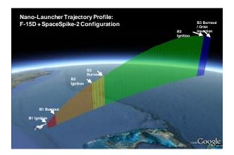
Figure 13. Orbital Nano-Launcher Preliminary Trajectory Profile: <u>F-15D + SpaceSpike-2</u> Configuration (to 250 km Circular LEO, 28.5 degree inclination launch site, release point off the coast of Florida)
