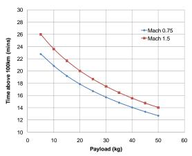
Figure 12. Suborbital Nano-Launcher Preliminary Payload Capability: <u>F-104 + two stage SpaceSpike-1</u>, Two Release Conditions: M=0.75 (at 9.144 km/30 kft) and M=1.50 (at 14.427 km/47.33 kft)
