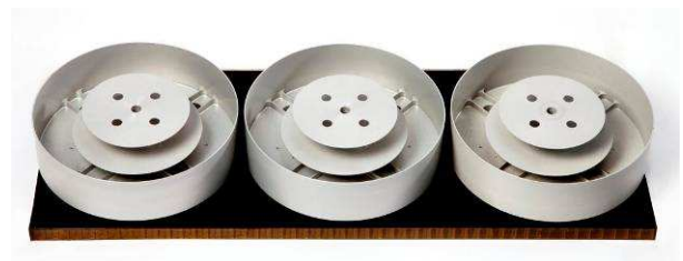
Figure 3: Three flight models of the PEC antenna without choke ring
