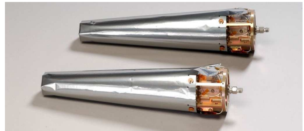
Figure 28: GPS helix antenna flight models with SLI cover
