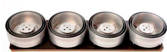
Figure 10: Four flight models of the PEC antenna with two choke rings
