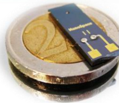
MEMS Isolation Valve
