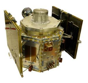
Figure 1. Phase 3 Bus with Payload Mass Simulator for Environmental Testing
