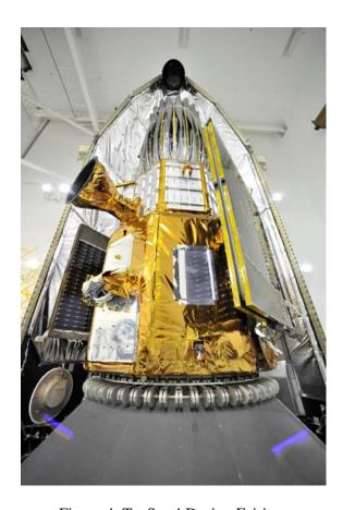
Figure 4. TacSat-4 During Fairing Encapsulation
