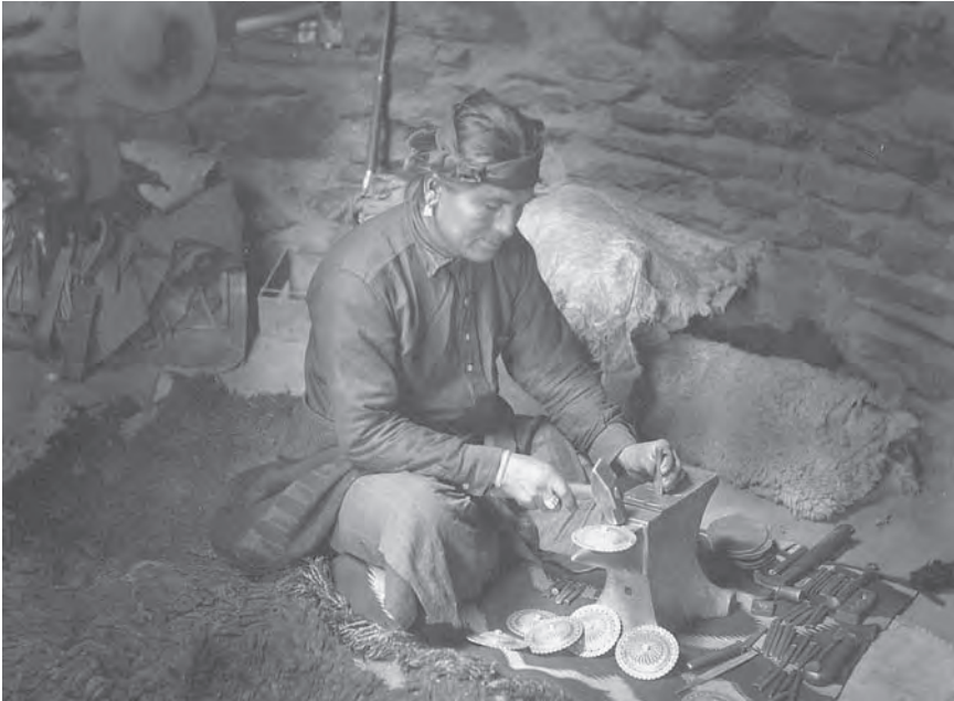
Navajo silversmith sits on a sheepskin with his tools. Finished silver conchos are on one side of the anvil and silver blanks on the other side. Photo by William Pennington.
