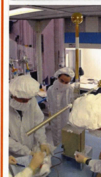
Above: SDL's Floating Potential Measurement Unit (FPMU) is a tool to study how the International Space Station charges as it flies through space.
